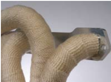
Remember when it comes to exhaust wrap, overlapping 1/4" is perfect as this allows just enough heat out to ensure performance without damaging your exhaust.
